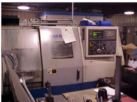
Newer machines usually have doors and guarding that cover the working parts of the machine tools. These are effective in isolating the operator from the MWFs. Older equipment does not have these controls and splash guards may need to be fabricated to shield the operator from MWF splashes. Other controls include:
