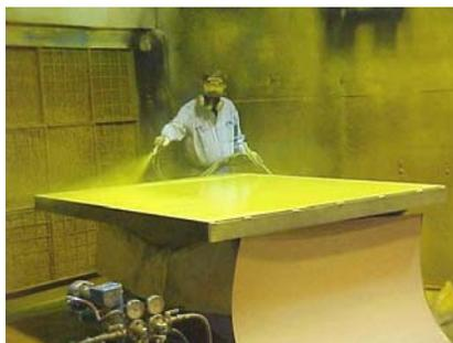
This figure shows an employee standing between the work piece and the exhaust of the booth. This results in overspray blowing back toward the operator. If the booth is shallow, overspray may also be blown out of the booth.
