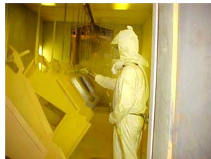
This figure shows an employee applying powder coat paint inside a paint booth wearing a supplied air hood.
