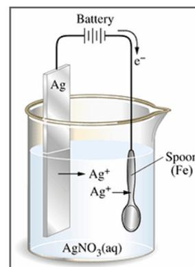
If the anode is an inert electrode, the bath is maintained by periodically adding metallic salts of the desired metal to the bath.
