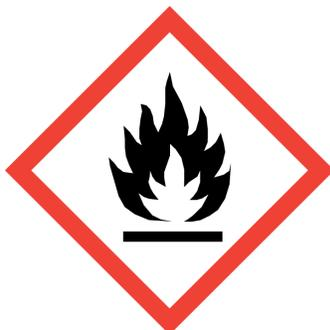
The GHS (Global Harmonized System) definitions are now used on labels and in SDSs. There are four categories of flammable and combustible liquids under GHS.
